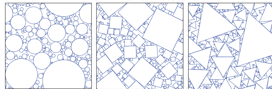
Physicists study random Apollonian packings as a model for foams or powders. In these simulations, new bubbles or grains nucleate in a random place and grow, either with rotation or without, until they encounter another bubble or grain. Different geometries for the bubbles or grains, and different growth rules, lead to different values for the dimension of the residual set—a way of measuring the efficiency of the packing. (Image courtesy of Stefan Hutzler and Gary Delaney.)
